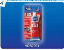
makes reliable "formed-in-place" gaskets that resist cracking, shrinking and migrating caused by thermal cycling. Hence ideal for use as replacement for gaskets, seals, gasket dressings, cork, felt, paper, rubber and asbestos gasket. It is permanently flexible and stable at temperatures from -80°F to 650°F (-62°C to 343°C). It is also highly resistant against oil, transmission fluid, water and antifreeze
