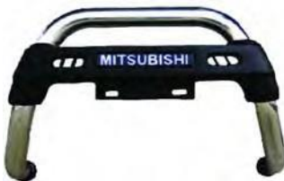
STAINLESS STEEL TUBE FRAME CENTER PLASTIC GUARD
